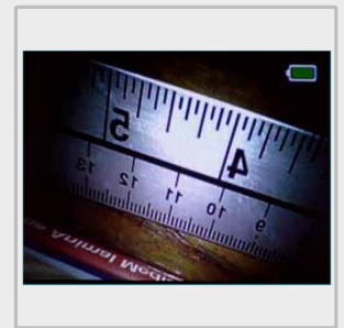
Mirror image function that allows 180° switch for clear analysis.
