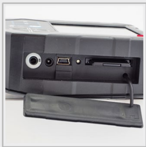
Easy access to interface: USB Port, power, SD Card Slot.
