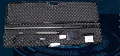
1 IP65 P&T camera white LEDs or IR 940NM with talk back function - 1 touchscreen monitor 7.0" - 1 HDMl cable - 1 AC charger - 1 USB Cable - 1 SD Card 32 GB - 1 rugged carrying case - 1 instruction manual - 1 cleaning kit BIPOL.
